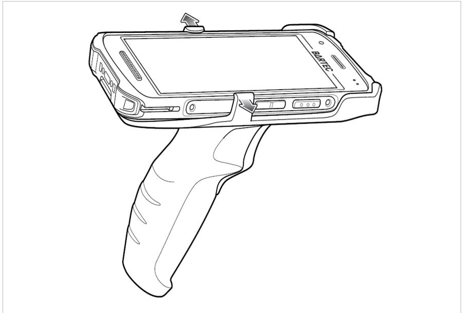
3. Rotate the bottom of the device up.
