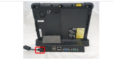
2. Plug the standard non-Ex USB stick with the operating system into a USB port of the docking station.
