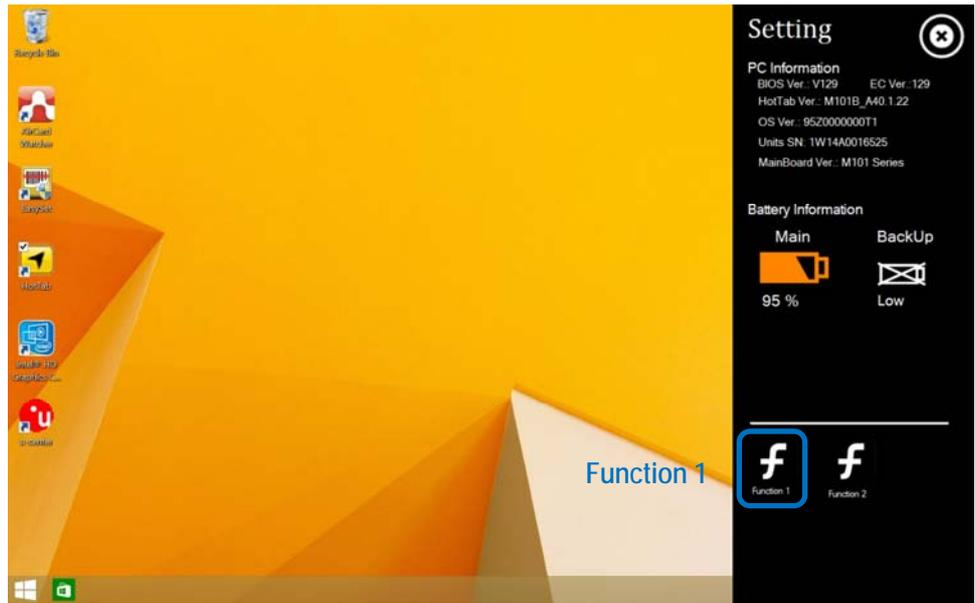
Select "Function 1" and you open the menu for setup of the function key.
