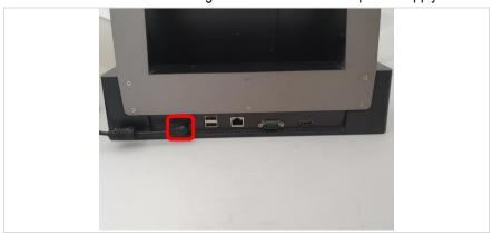
2. Plug the Bartec Ex-i USB stick with the operating system into the USB port of the Tablet-PC.
