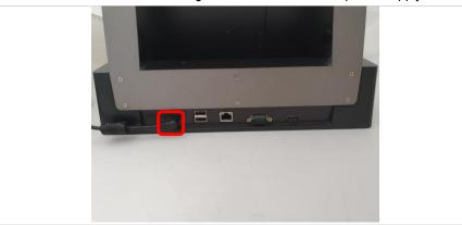
2. Plug the standard non-Ex USB stick with the operating system into a USB port of the docking station.
